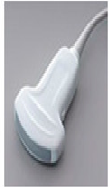
5-2 MHz 60-mm curved array
